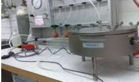
Test on valves of coffee packaging
