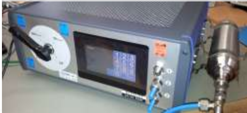
Calibration device for reviewing test leaks
