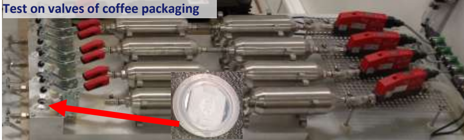
Calibration device for reviewing test leaks
