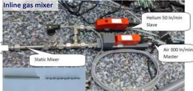
Master channel Thermal mass flow meter GSM 4 – 400 l/min Ar at 8 bar g
