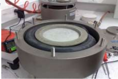
Permeability test of membranes
