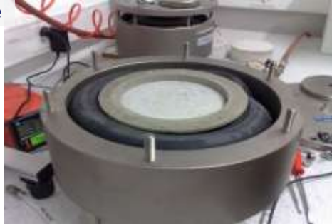
Permeability test of membranes
