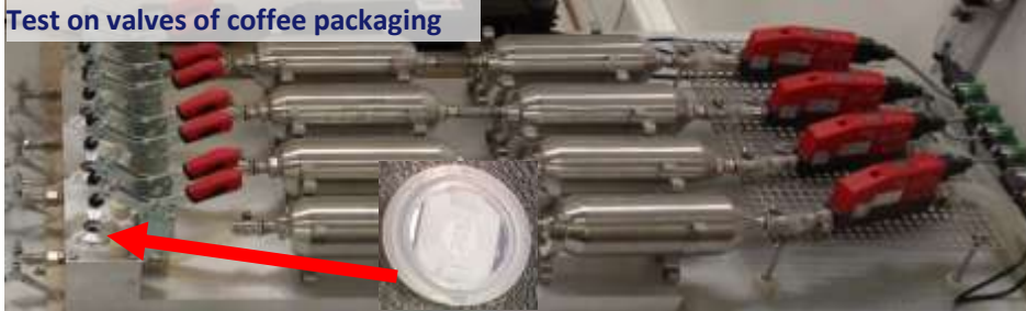
Calibration device for reviewing test leaks
