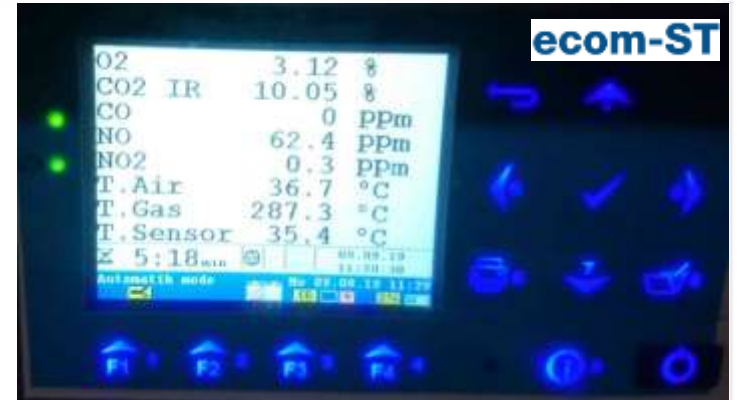
Flue gas analyzer display in operation
