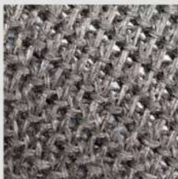
A microweave mat made from a high-quality alloy permits the right amount of gas/air mix to pass
