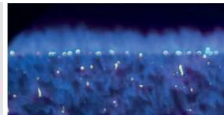
The homogeneous mixture of gas and air combusts on the surface of the woven metal mesh at temperatures < 1200 °C. This combustion technology effectively inhibits the formation of thermal NO x .
